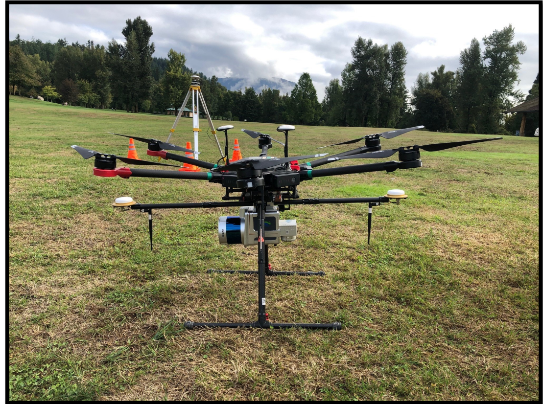
Drone with LIDAR attachment used for surface mapping of the grounds of the second St. Mary's institution (Fraser River Heritage Park). Photo: Dave Schaepe
